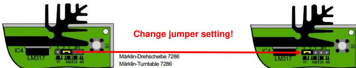
2. For **Märklin and Fleischmann** turntables with sb drive, the speed must be reduced and the control cycle adjusted.
