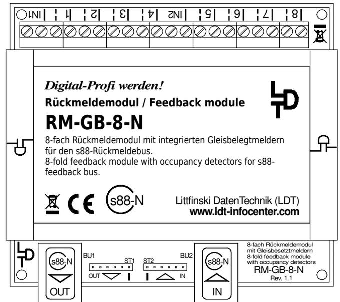
The **track voltage** and the **feedback bus** are separated by **opto-galvanic**. The current for the tracks can therefore safely be supplied from different transformers without having a negative effect on the digital control units.
