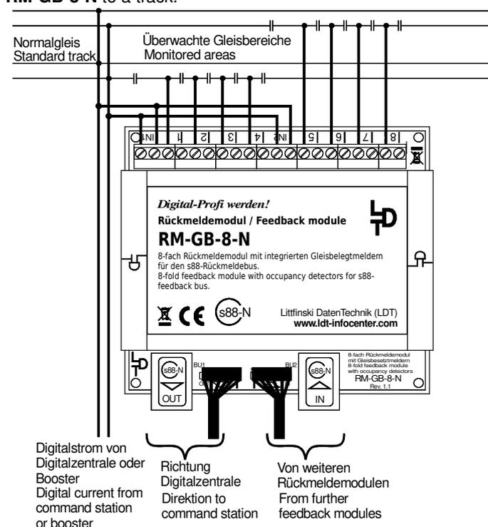
Digital current will be supplied to the **RM-GB-8-N** via input **IN1** and **IN2**. **IN1** provides current to the output **1** to **4** and **IN2** provides current to the output **5** to **8**. The two inputs **IN1** and **IN2** are **electrical separated**.
