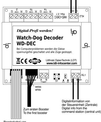
Boosterkabel von der Steuereinheit (Zentrale) Boostercable from command station (central unit) Please attend to the marking on clamp KL1.
