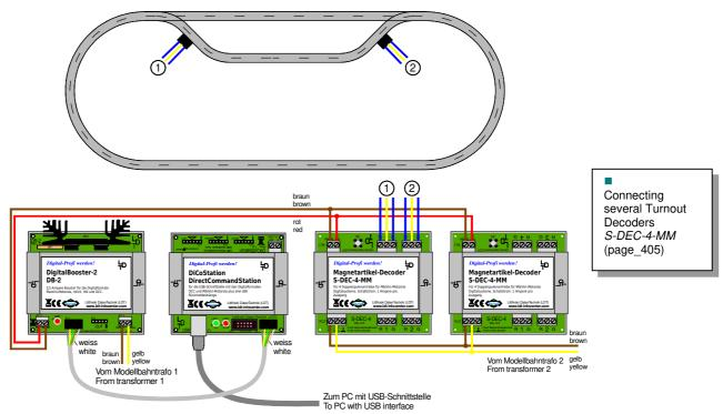
It is recommended to install a separate second main ring conductor for the digital current to the turnout- and switch decoders (**red** / **brown**) and a third main ring conductor for the voltage supply (**yellow** / **brown**).
