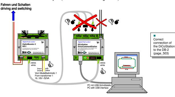
For the power supply to the Booster "DB-2" we recommend to use a model-railway-transformer with 16 to 18 Volt alternated voltage and a capacity of a minimum of 52VA.
