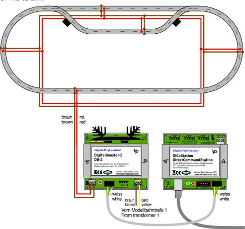
Rail ring conductor with supply connections (page\_404)
