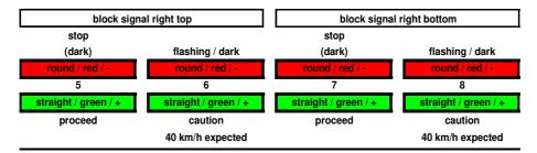
After switching-on the layout the Light-Signal Decoder switches both block signals at first to red (stop).
