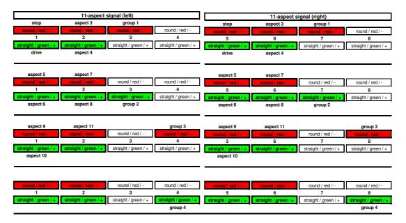
For indicating e.g. at the right signal the aspect 9 it is required at first to activate the address 8 key **Red** for the third signal aspect group and then the address 5 key **Red**. At the sample has been the four-fold address group 5 to 8 assigned to the signal at the right clamp bar.
