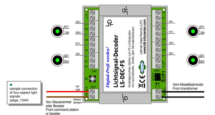
The signals connected to the left side occupy e.g. the decoder addresses 1 to 4. The addresses 5 to 8 will be used by the right signals. Each signal occupies therefore 2 decoder addresses and all signals can be switched independently.
