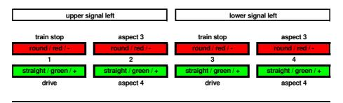
To switch e.g. the lower signal of the right clamp bar to green (drive) you have to activate the **green** key of the address 7. The following table shows the setting of keys and the assignment of digital addresses:
