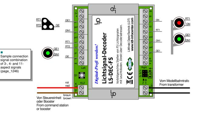
The 3-aspect signal will be exemplary controlled via the two addresses 1 and 2. The 4-aspect signal will be controlled via the addresses 3 and 4.
