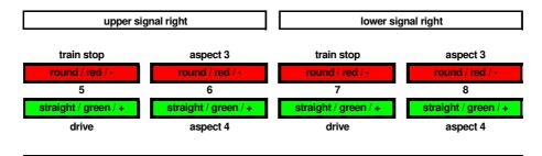
The following sample connection shows the digital control of four 3-aspect signals by the Light-Signal Decoder *LS-DEC-FS*:
