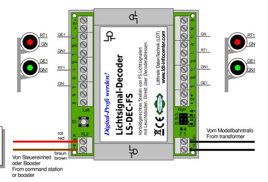
sample connection 11-aspect light signals (page\_1245) The following key-occupancy shows the relation for the two connected 11-aspect signals.
