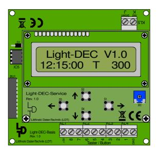
The universal Layout-Light-Control Light-DEC consist of one Basic-Module and as minimum of one Light-Module (Light-Display or Light-Power) which has to be plugged onto the side of the Basic-Module.
