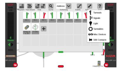
Under "Type" select "Scale Color Light Signal HP0/1/2+SH0/" for the main signal.
